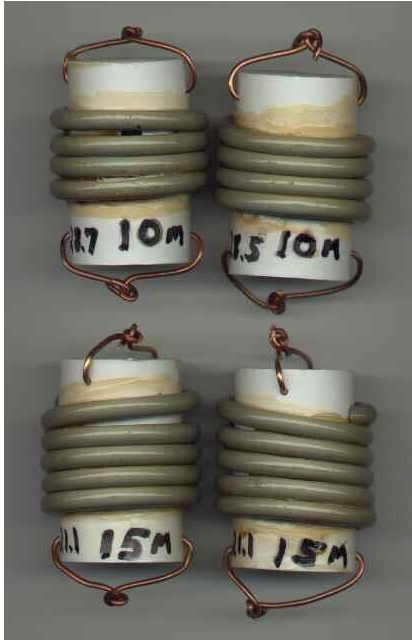
The 10 and 15 meter traps, wound on 3/4" PVC pipe couplings.
