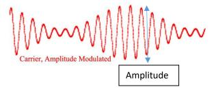
**Modulation:** The mixing of voice (intelligence) with a single frequency wave usually of radio frequencies (the carrier). There are major types, amplitude modulation and frequency modulation. In AM, the amplitude of the carrier is changed and in FM the frequency is increased and decreased to encode the volume of the voice.
